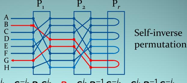
$$Q = S^{-i_1} P_1 S^{i_1} \cdot S^{-i_2} P_2 S^{i_2} \cdot P_r \cdot S^{i_2} P_2^{-1} S^{-i_2} \cdot S^{i_1} P_1^{-1} S^{-i_1}$$
