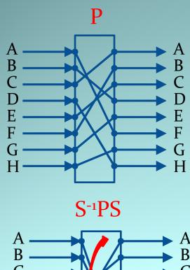
P = Permutation embedded in rotor
