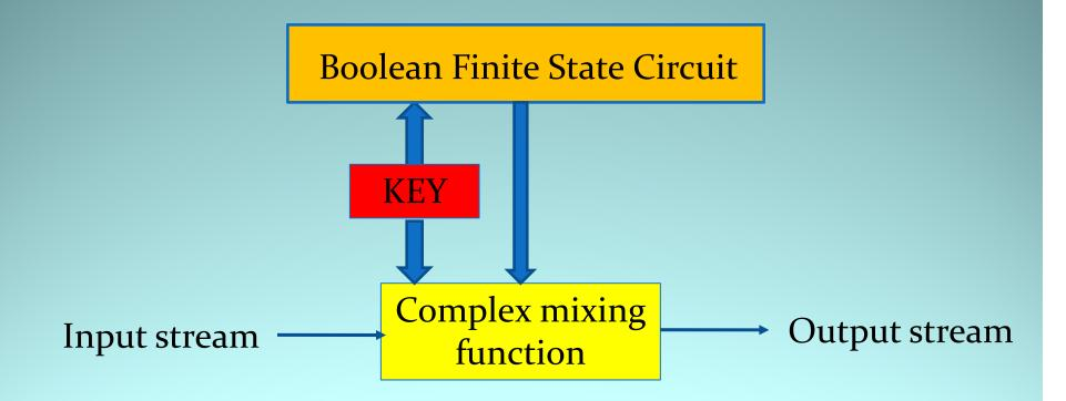
Stream cipher with a dynamic key-dependent mixing function
